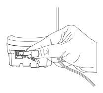
5. Place the cord inside the molded channel on the bottom of the Base Unit.
